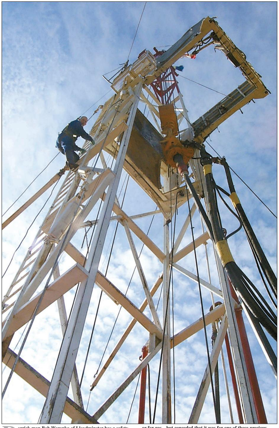
errick man Bob Werenka of Lloydminster has a safety strap attached to his body as he climbs a drilling rig a half mile north of Highway 13 and east of Metiskow.
